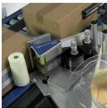
No need to split lines - the 9550 can direct print and apply labels
